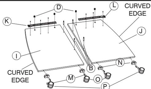
Brackets to the bottom edges of the Side Panels (caster sockets should be on the same side as the Panel holes.)
